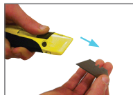
3. Carefully remove blade
